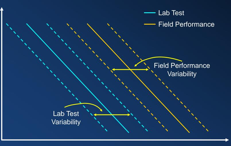
Cycles to Failure
