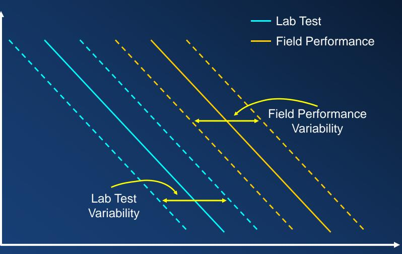
Cycles to Failure
