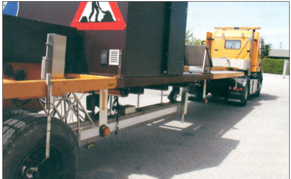
The High Speed Deflectograph developed by the Danish Road Directorate
