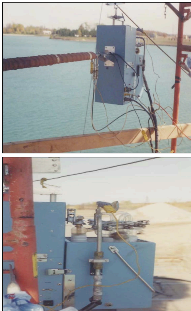
Figure 9: Dry ice trap for sampling at the stack.
