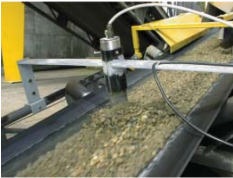
Microwave moisture probe on the conveyor belt
